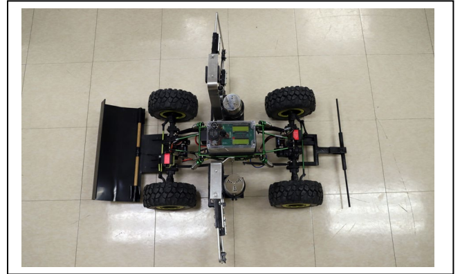
Fig. 5. Rover with fabric wings and drag mat removed for clarity. The robot’s front is to the left of the image. The magnetic field sensors are attached on either side of the front vegetation plow. A suspension system including shock absorbers help it navigate hilly terrain. The weather-proof box containing both PCBs can be seen on top of the rover, between the two wings. The battery compartment is directly beneath this holder. The spring-loaded wings on both sides and the drag bar in the rear will hold fabric squares that have been sprayed in permethrin; ticks will attempt to attack these areas, and in seconds will absorb a lethal dose of permethrin.
