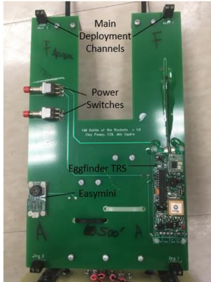
Figure 3. Completed printed circuit board with the two flight computers, electrical connections for the e-match ejection charge ignitors, and separate disconnect switches labeled.
