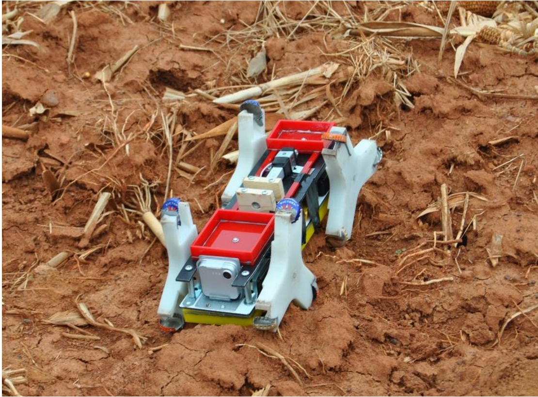
Figure 4. Mars Rover staged in a cornfield for a full systems test. The whegs rotate together for horizontal movement and then counter-rotate, causing the bottle-tops to scoop dirt into angled channels in the whegs that ultimately deposit it into the red top-mounted trays. The system is vertically symmetric; should the rover land upside-down it will work in the same manner. The camera is visible at the front and the parachute-detachment mechanism in the rear.
