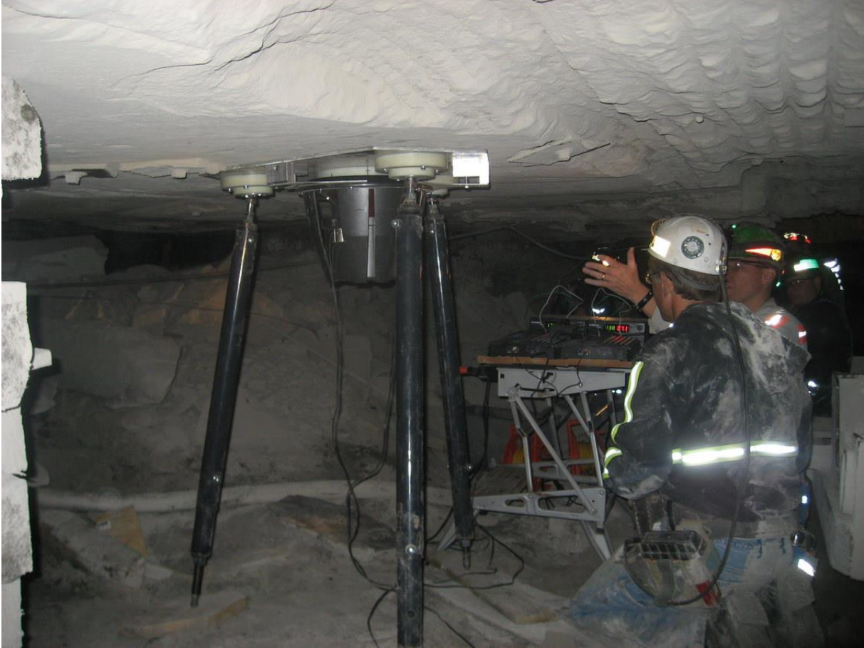
Figure 4: Profs. Squire and Sullivan set up the 12 th generation of the VMine in a commercial mine in Tennessee under the watchful eyes of a federal MSHA safety representative. The tests demonstrated that the VMine could communicate in the deepest typical east coast mines, and shortly after the team licensed the device to a major mine safety equipment manufacturer.
