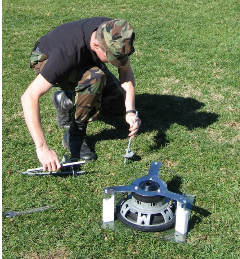
Figure 2: Cadet Will Flathers sets up a fourth-generation version of the VMine on the parade field at the Virginia Military Institute. It many design iterations before the team developed a prototype that worked at depths of typical mines.
