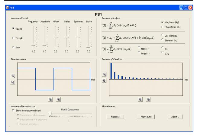
Figure 1: The Fourier Synthesis application program
