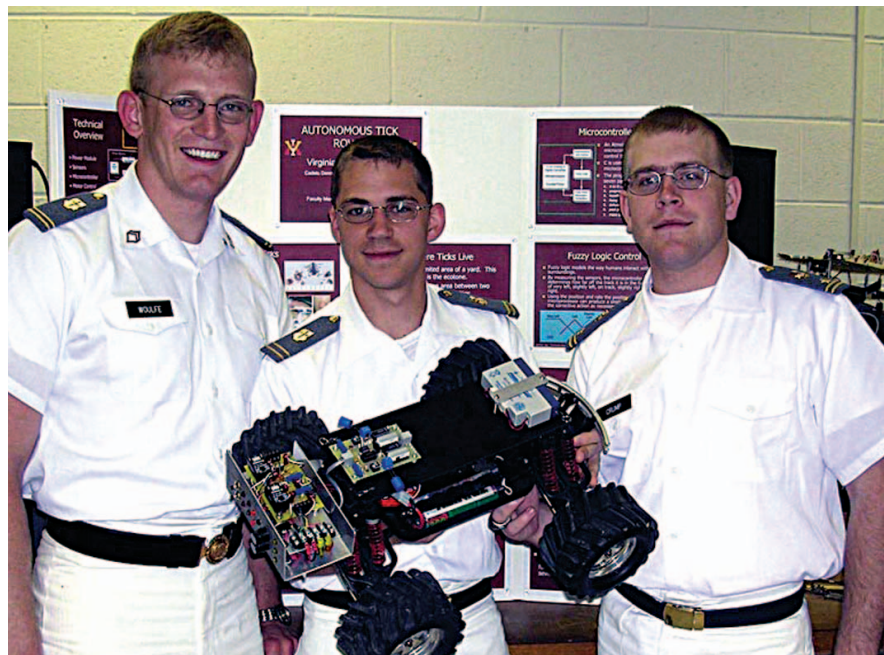
Fig. 1 The authors and the tick-collecting robot. The power supply is visible at the rear of the vehicle; the micro controller and sensor PC boards are in the center. Not shown is the fabric skirt that the ticks naturally adhere to or the chemoattractant tube/navigation wire that draws the ticks to a narrow region and provides a signal for the rover to follow.
