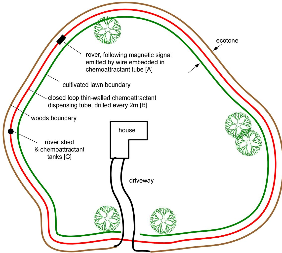
Figure 1: The tick rover (A) follows a signal from the wire (B) to follow the ecotone around a home's perimeter. Coaxial with the wire is a tube drilled to dispense a tick chemoattractant. The rover pauses in a shed (C) every lap to recharge and self-clean.
