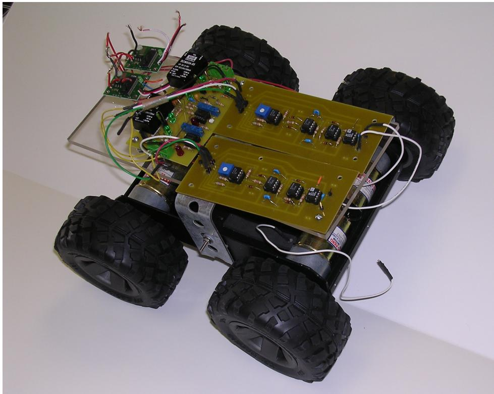
Figure 2: The Phase I prototype is shown. The two symmetric sensor boards are mounted in front of the power module. The motor controllers are mounted in the rear. All five units are secured on a clear piece of Plexiglas. The charging lead can be seen in the front of the rover
