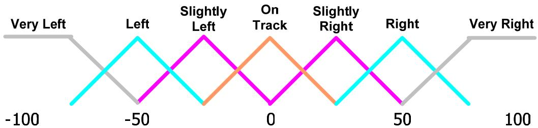
Figure 5: Fuzzy sets used in the robot controller which correspond to the distance of the wire from the center of the rover. The farther the distance from the center, the larger the corrective action instruction given by the controller.
