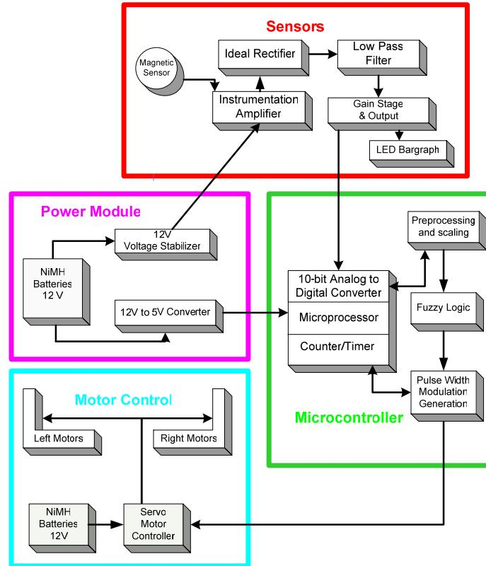
Figure 4: Block diagram of the high level design of the rover. The sensor data is processed by the microcontroller which instructs the motor controller to take the necessary corrective action to stay on track.
