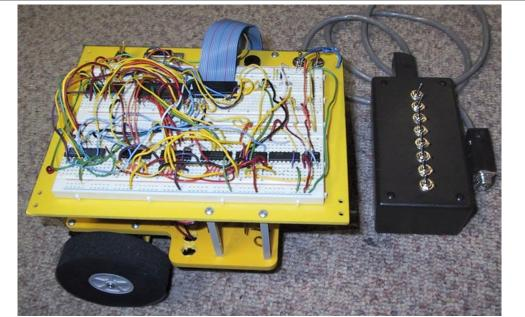
Figure 1: The custom robot base used at VMI. Students add soldered PC boards that they assemble (e.g. an H-bridge motor controller and contact sensors) to the frame, and build the digital logic on the supplied solderless protoboard. The teaching pendent used for programming is shown to the right.
