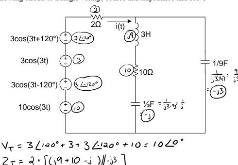
$$V_{\tau} = 3 \angle 120^{\circ} + 3 + 3 \angle 120^{\circ} + 10 = 1020$$
