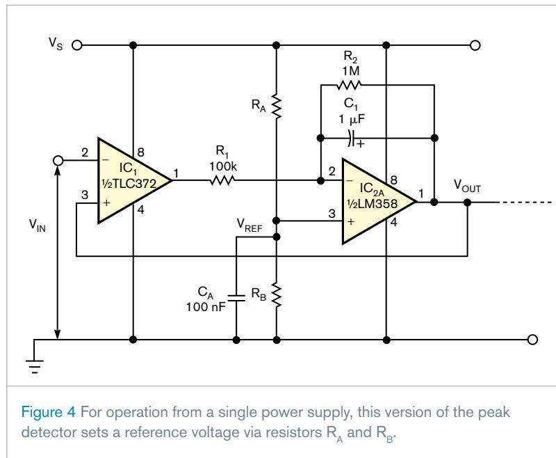
**Figure 4** For operation from a single power supply, this version of the peak detector sets a reference voltage via resistors  $R_A$  and  $R_B$ .
