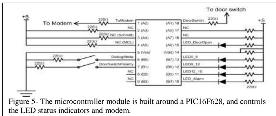
Figure 5- The microcontroller module is built around a PIC16F628, and controls the LED status indicators and modem.
