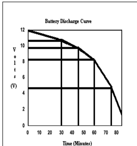
Figure 4: Experimentally-measured battery voltage discharge curve, showing the location of comparator trip points at voltages corresponding to 90, 45, 30, and 15 minutes remaining.
