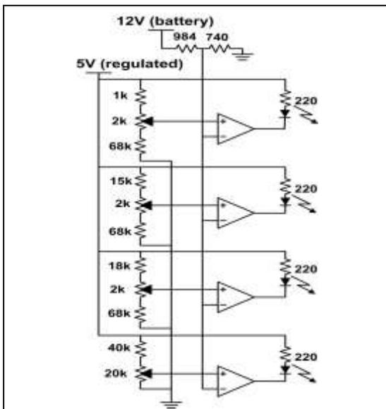
Figure 3: The battery strength module displays whether the battery can power the refrigerator and electronics for 90, 45, 30, or 15 additional minutes.
