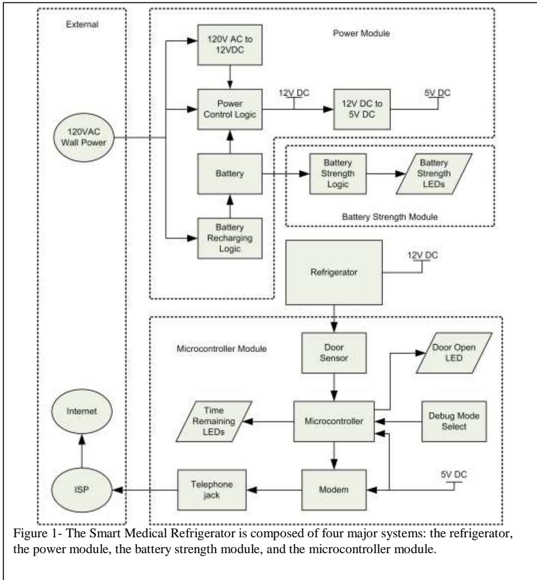
Figure 1- The Smart Medical Refrigerator is composed of four major systems: the refrigerator, the power module, the battery strength module, and the microcontroller module.
